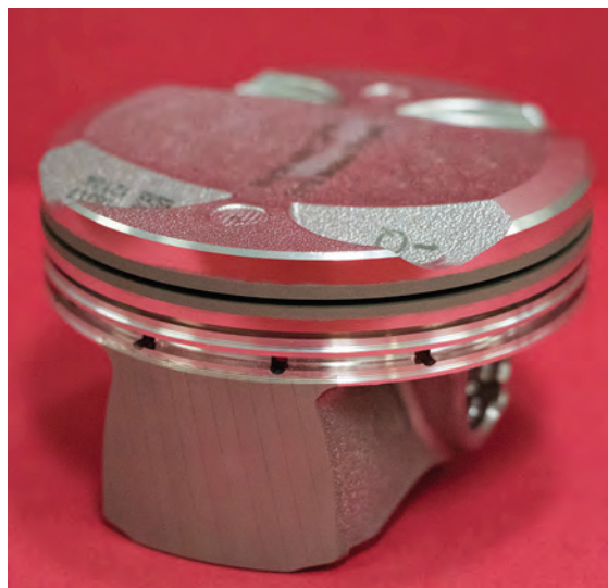
A car engine piston off the production line of a large auto manufacturer is shown; the piston has been treated with a femtosecond laser for enhanced engine performance.
